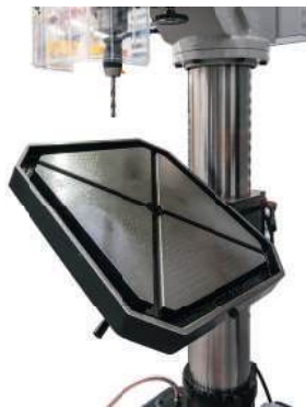
MESA GIRATORIA INCLINABLE TILTING ROTARY TABLE
