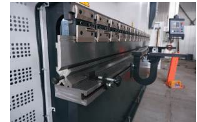
Amarre Sistema Promecam CLAMPING SYSTEM PROMECAM
